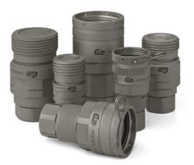
TLX is a Flat-Face twist lock coupling for the toughest applications in the construction and demolition segment. This super-duty quick connect coupling is designed to work with the highest surge flows and the toughest pressure impulses. TLX is made from high alloy steels with Zinc-Nickel surface treatment for a long life in the harshest conditions. The Series is available in sizes from <sup>3</sup>/<sub>4</sub>" to 1 <sup>1</sup>/<sub>4</sub>" to cover most applications.
