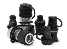
Series 125 is a CEJN original with extremely small outside dimensions and a patented seal design, making it ideal for bolt tensioners, bearing pullers and other applications. All exposed components are made of zinc-plated steel. Like all products featured in the CEJN High-Pressure range, non-drip connection and disconnection are standard. Plastic dust caps are also standard on the couplings and nipples, a feature that extends the service life of the entire hydraulic system.
